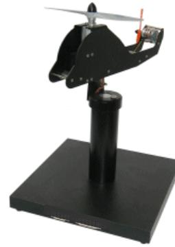
**Fig.4 Model 'helicopter' (Humusoft Co.)**
