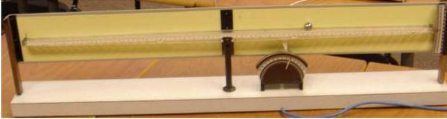
**Fig.1 Laboratory model 'ball on rod'**
