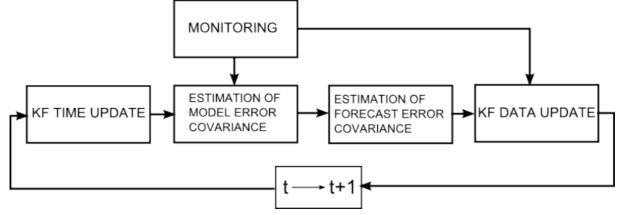
Figure 1. Schematic of one cycle of recursive assimilation algorithm.
