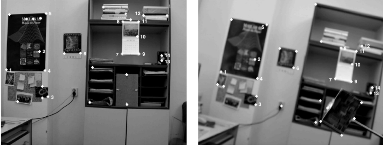
Fig. 8. Images of the indoor scene. Camera at the initial position (left); camera at an unknown position, the scene is out-of-focused due to the inserted object (right). 30 CPC's are marked by crosses, those which form the corresponding CP pairs are numbered.
