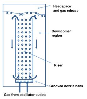
Fig. 7 – Schematic diagram of an internal ALB with draught tube configured with a tailor made grooved nozzle bank fed from the two outlets of the fluidic oscillator. The microbubble generator is expected to achieve nearly monodisperse, uniformly spaced, non-coalescent small bubbles of the scale of the drilled apertures.
