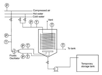
Fig. 8 – Process flow diagram of the airlift bioreactor gas separator.
