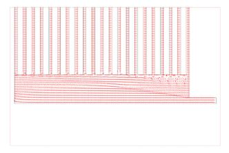
Fig. 10 – Flow field within the distributor when a pressure gradient of 10 Pa applied across it. A negative pressure develops near the inlet.
