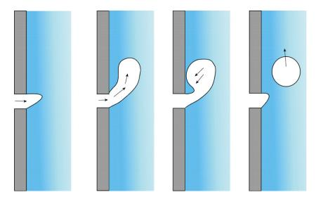
Fig. 6 – An schematic of the microbubble generation from a horizontally oriented nozzle/gas flow path. There are four distinct phases: (1) pushing out of a hemispherical cap at the beginning of the upstroke of the fluidic oscillator; (2) buoyant rise of the growing bubble during the remainder of the upstroke; (3) suction of the bubble to collide against the solid surface; (4) recoil of the bubble from the solid surface and breakoff of the bubble.
