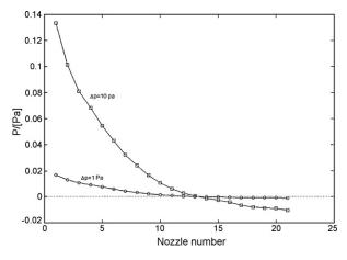
Fig. 11 – Pressure distribution in the nozzle manifolds. Nozzle count is from left to right (of the arrangement shown in Fig. 10). The negative pressure is due to the nozzle effect at the inlet area.
