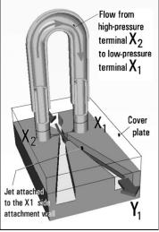
Fig. 2 – Left: the model of the fluidic jet-deflection amplifier used in the tests. It is a stack of PMMA plates with laser-cut cavities – containing no moving mechanical parts. The screws are 1/4 inch heads. Right: the fluidic oscillator is made from the amplifier by providing it with the feedback loop (shown here of adjustable length for tuning the oscillation frequency) connecting its two control terminals.
