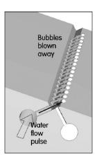
Fig. 4 – Left: configuration for the blow-off mechanism for bubble detachment. While the same diverter oscillator as in Fig. 3 is used, only one of its outputs, A, is used to deliver the air to the aeration apertures during the half-period. The other, B, delivers a water flow pulse into a system of adjacent water-flow nozzles. Centre: the bubble formation half of the period. Right: water flow pulse removes the nascent bubbles from their apertures.
