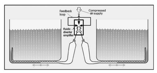
Fig. 3 – Schematic representation of the fluidic diverter oscillator driving the microbubble generation system with two nozzle banks fed by alternate oscillation "strokes".
