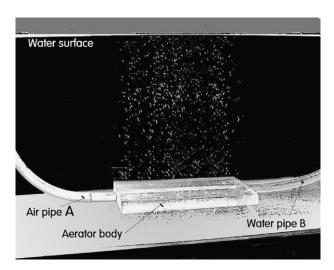
Fig. 5 – Tiny bubbles generated in an experiment with the aerator system model corresponding to Fig. 4. Actually, the same nozzle bank is used as the one generating the large bubbles with the steady (non-oscillated) air flow through the 0.6 mm holes as shown in Fig. 1.
