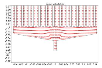
Fig. 12 – Flow field within the distributor when the inlet is place at the centre parallel to the nozzle manifolds. Pressure gradient across the distributor is 10 Pa.
