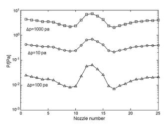
Fig. 13 – Pressure distribution in the nozzle manifolds for the geometry shown in Fig. 12. Nozzle count is from left to right.
