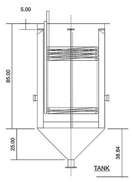
Fig. 9 – The design of the bioreactor (dimensions are centimeters).
