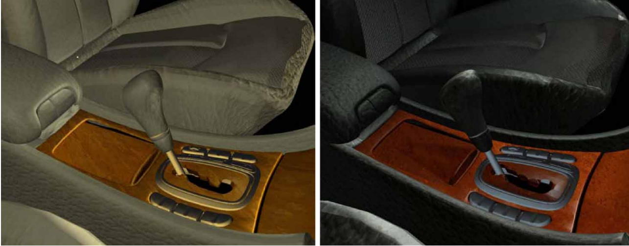
Figure 12. A screen-shot from a UTIA real-time BTF rendering application of the car interior using the proposed BTF enlargement technique (3D CAR) applied to lacquered wood materials on the upper console of the gearbox.
