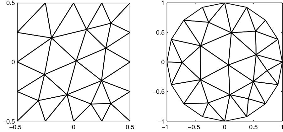
Figure 1: The meshes used for the first (left) and the second (right) test problem.
