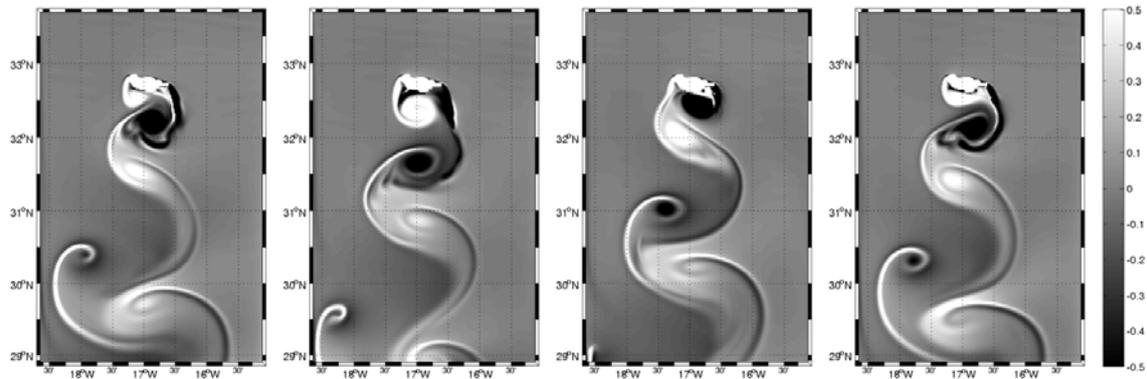
Figure 2. Time varying shedding for 30th, 35th, 40th and 45th model days (from left to right). Colours represent surface vertical vorticity.
