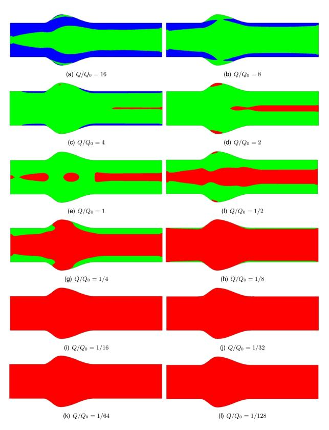
Figure 2: Relative viscosity magnitude,  $\bar{\eta} = (\eta(\dot{\gamma}) - \eta_{\infty})/\eta_{\infty}$ , aneurism geometry
