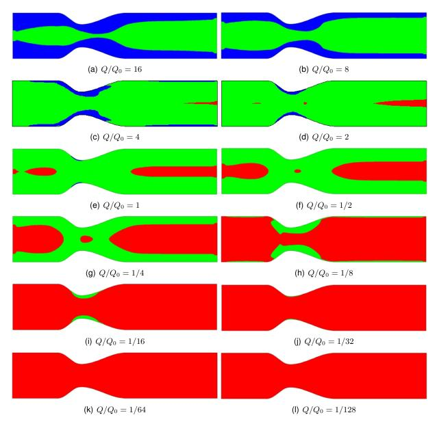
Figure 1: Relative viscosity magnitude,  $\bar{\eta} = (\eta(\dot{\gamma}) - \eta_{\infty})/\eta_{\infty}$ , stenosis geometry
