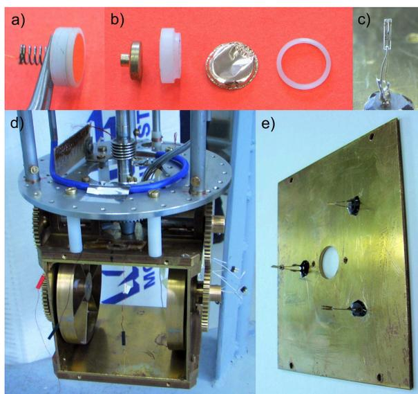
Obrázek 1: An assembled (a) second sound sensor based on the gold-plated nuclepore membrane, mechanically stretched over a delrin ring, forming a capacitor with the opposite brass electrode (b) pressed against it by a spring. Detailed view of one of the bare quartz tuning forks sealed with Stycast 1860 to the brass wall (c) and the geometric configuration (e) of three forks. The photograph of the lower part of the cryogenic insert showing the brass cell (d).
