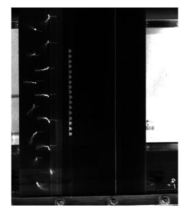
*Fig.* 5 non-controlled case, 0deg deflected flap,  $\alpha = 15^{\circ}$
