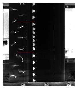
Fig. 4 rectangular VG (h=3mm,  $\Delta z$ =16mm, red lines area), 20deg deflected flap,  $\alpha = 0^{\circ}$
