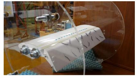
Fig. 1 Position of VGs on NACA 63A421 airfoil
