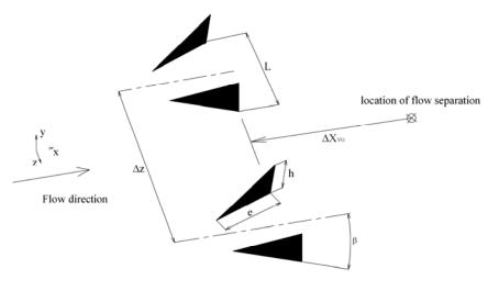
Fig 2 VGs design and its relative position
