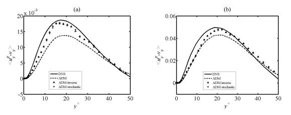
Figure 1: Mean relative velocity (a) St=1 and (b) St=5.
