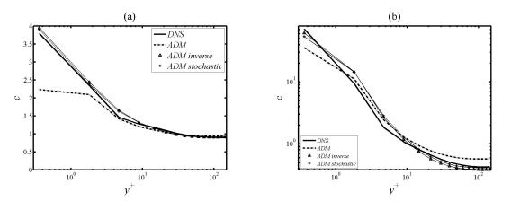
Figure 4: Concentration of particles close in the stationary state for (a) St=1 and (b) St=5
