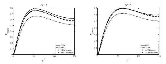
Figure 2: Wall-normal particle velocity fluctuations for St=1 and St=5.
