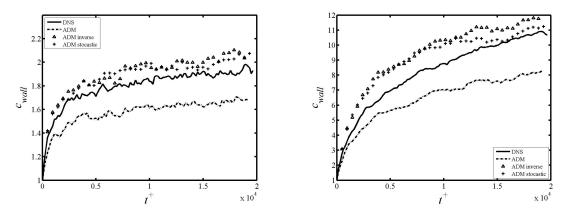
Figure 3: Concentration of particles close to the wall as a function of time for St=1, St=5.
