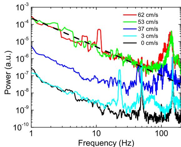
Obrázek 2: Energy spectra in He I as detected by the piezoelectric pressure sensor. The bottom line shows the spectrum measured with discs at rest; other spectra correspond to ascending velocities as indicated. The dashed line illustrates the Kolmogorov roll-off exponent of  $-5/3$ .
