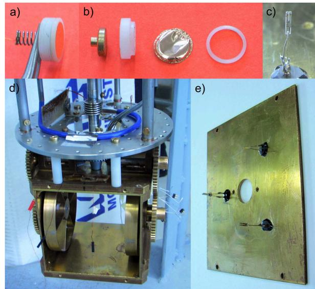
Obrázek 1: An assembled (a) second sound sensor based on the gold-plated nuclepore membrane, mechanically stretched over a delrin ring, forming a capacitor with the opposite brass electrode (b) pressed against it by a spring. Detailed view of one of the bare quartz tuning forks sealed with Stycast 1860 to the brass wall (c) and the geometric configuration (e) of three forks. The photograph of the lower part of the cryogenic insert showing the brass cell (d).
