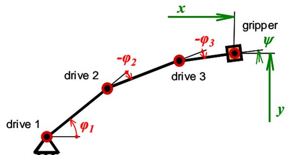
Fig. 1. Operational ( $x, y, \psi$ ) and joint ( $\varphi_1, \varphi_2, \varphi_3$ ) oriented coordinates (coordinate spaces)
