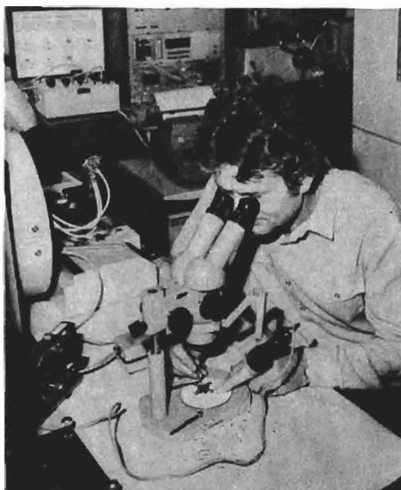
Setting up a special semiconductor transducer. Seen in the background a test rig for transducer calibration
