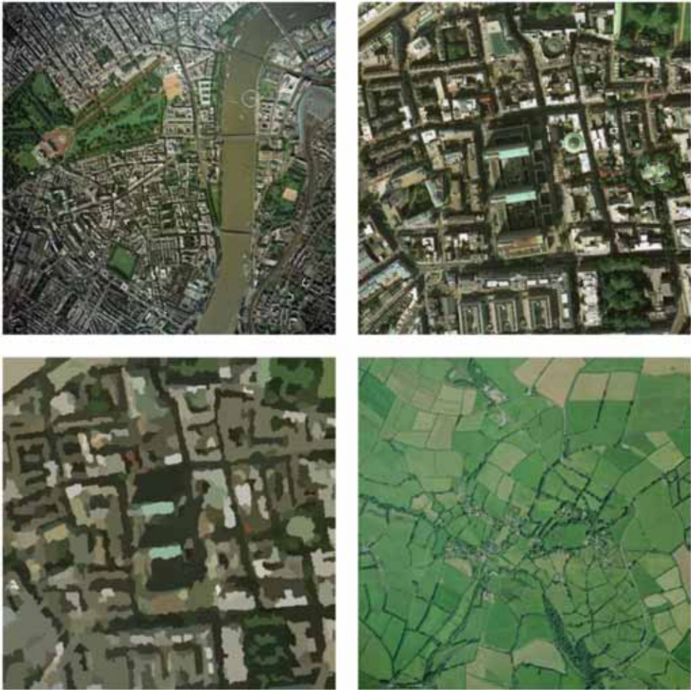
Fig. 7. Aerial Lmw 4800 \times 4800 image (top left), its detail (top right), the corresponding unsupervised segmentation (bottom left) and parrac 8000 \times 8000 image segmentation result, respectively.
