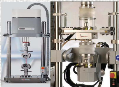
Mechanical testing laboratory, INSTRON ElectroPulse E3000 testing machine
