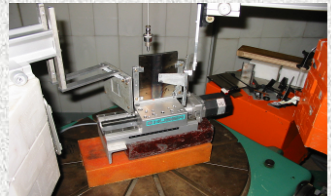
Neutron strain scanner for evaluation of residual stresses in engineering components
