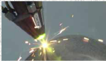
Direct Metal Deposition process by laser using TRUMP DMD equipment
