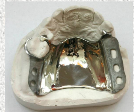
Removable partial dental parts made using 3D scanning advanced CAD and SLM (MCP Realizer)
