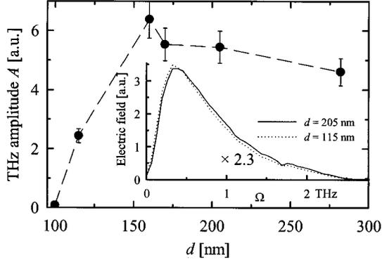
Fig. 1. Integrated THz pulse amplitude as a function of  $d$  with both the excitation and the THz beam  $p$  polarized; angle of incidence  $45^\circ$ . Inset, THz spectrum for  $d=205$  nm and  $d=115$  nm (linearly scaled).
