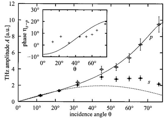
Fig. 2. Integrated THz pulse amplitude as a function of  $\theta$  for  $p$  and  $s$  polarization of excitation beam  $d=205$  nm. Inset, relative phase shift between the THz pulses in the two polarizations. Symbols, experimental data; curves, best fit using Eq. (1) for  $p$  polarization and Eq. (2) for  $s$  polarization.
