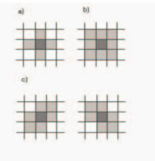
**Figure 1**: Definition of typical neighbourhoods which can be used in CA-simulations (a) von Neumann, (b) Moore, (c) hexagonal [5].
