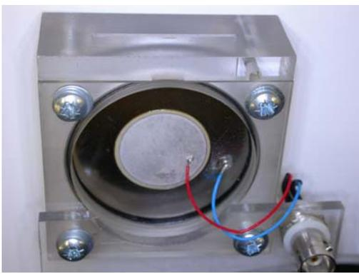
Fig. 2 – Synthetic jet generator
