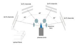
Figure 1. Experimental layout schematic.
