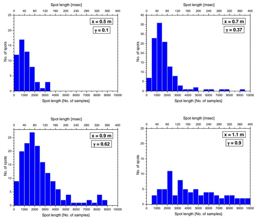
Figure 10 Number of spots as a function of spot length (for the coordinates  $x = 0.5, 0.7, 0.9$  and  $1.1$  m), GT-5,  $Le = 33.4$  mm.
