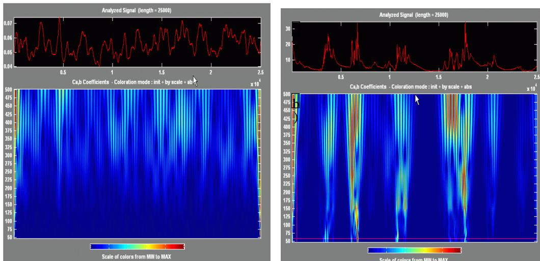
Figure 4 Morlet wavelet transforms of skin friction signal  $Tu = 0.03$ ,  $Le = 5.9$  mm: left:  $x = 0.1$  m,  $Re_1 = 318$ ,  $\gamma = 0$ : right:  $x = 1.0$  m,  $Re_1 = 921$ ,  $\gamma = 0.52$ .
