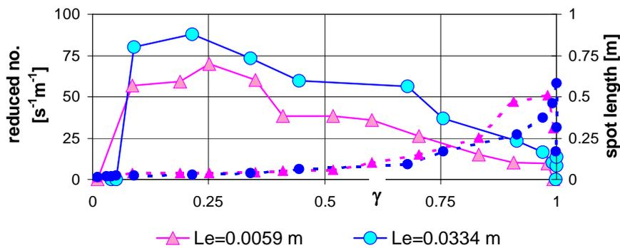
Figure 12 Reduced number and mean length of the identified turbulent regions versus intermittency factor (marks as in Figure 11)
