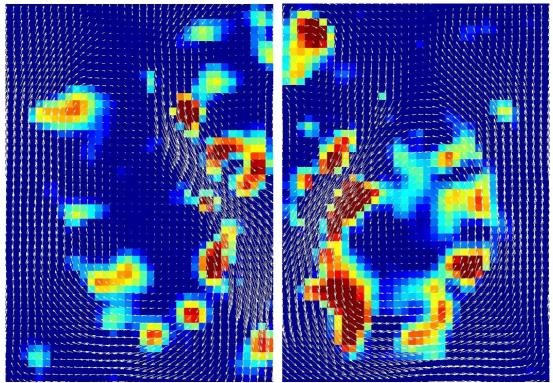
Fig. 1: The instantaneous flowfield with visualized vortical structure; the Kelvin- visualized vortical structure; the vortex loop just Helmholtz instability is clearly visible formed
