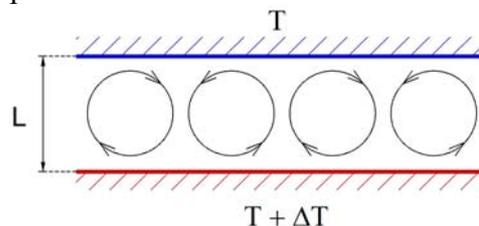
Figure 1: Schematic representation of Rayleigh-Bénard convection
