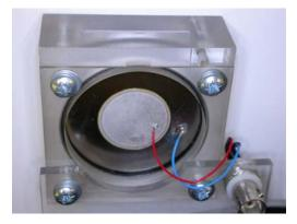
Fig. 2 – Synthetic jet generator
