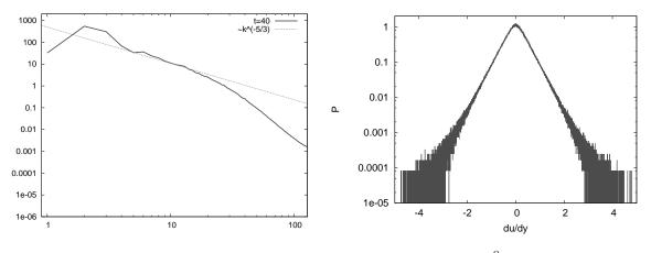
Figure 1: a) The energy spectrum at t = 40, b) A PDF of  $\frac{\partial u}{\partial u}$ .
