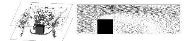
Figure 2: a) A snapshot of visualized vortices behind the cube, b) An averaged flow field in a xz plane of symmetry.
