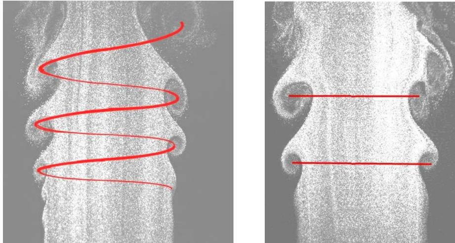
**Fig. 5 (Left)** Early experiments performed at the University of Sheffield (Tesař, Zimmerman, Regunath [8]) - visualisations of smoke-laden air jet by means of the laser light-sheet "knife". This picture demonstrates spontaneous formation of helical structures in the jet mixing layer.
