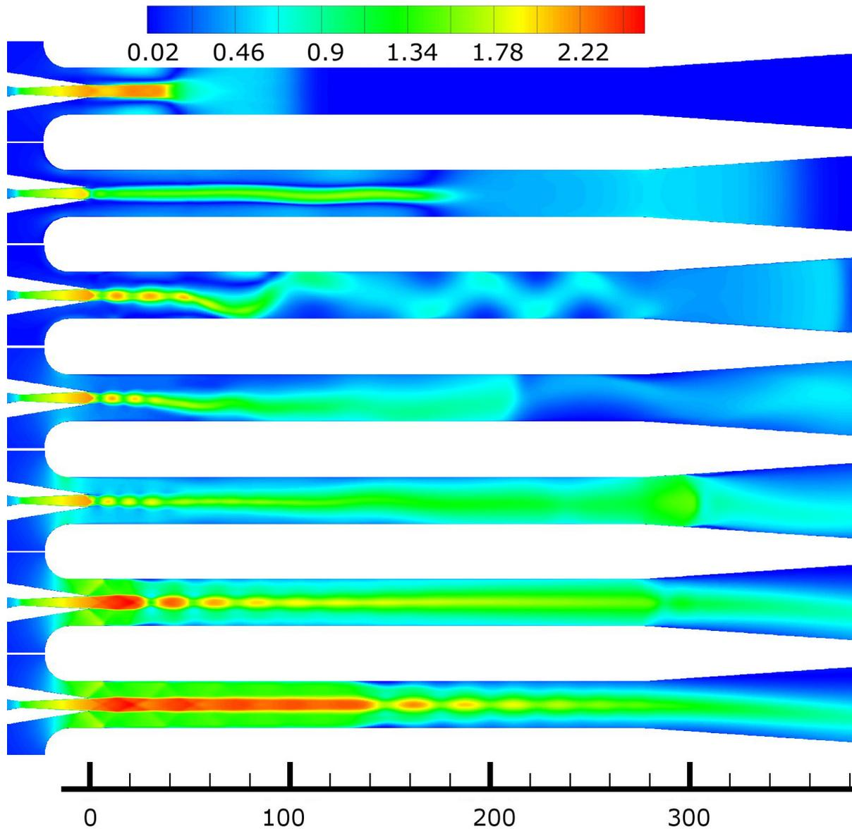
Figure 2: Evolution of the flow in the ejector (selected iterations), Mach number distribution,  $p_{01}/p_{02} = 4.09$ ,  $p_{02}/p_b = 1$ ,  $k - \omega$  model (Kok)
