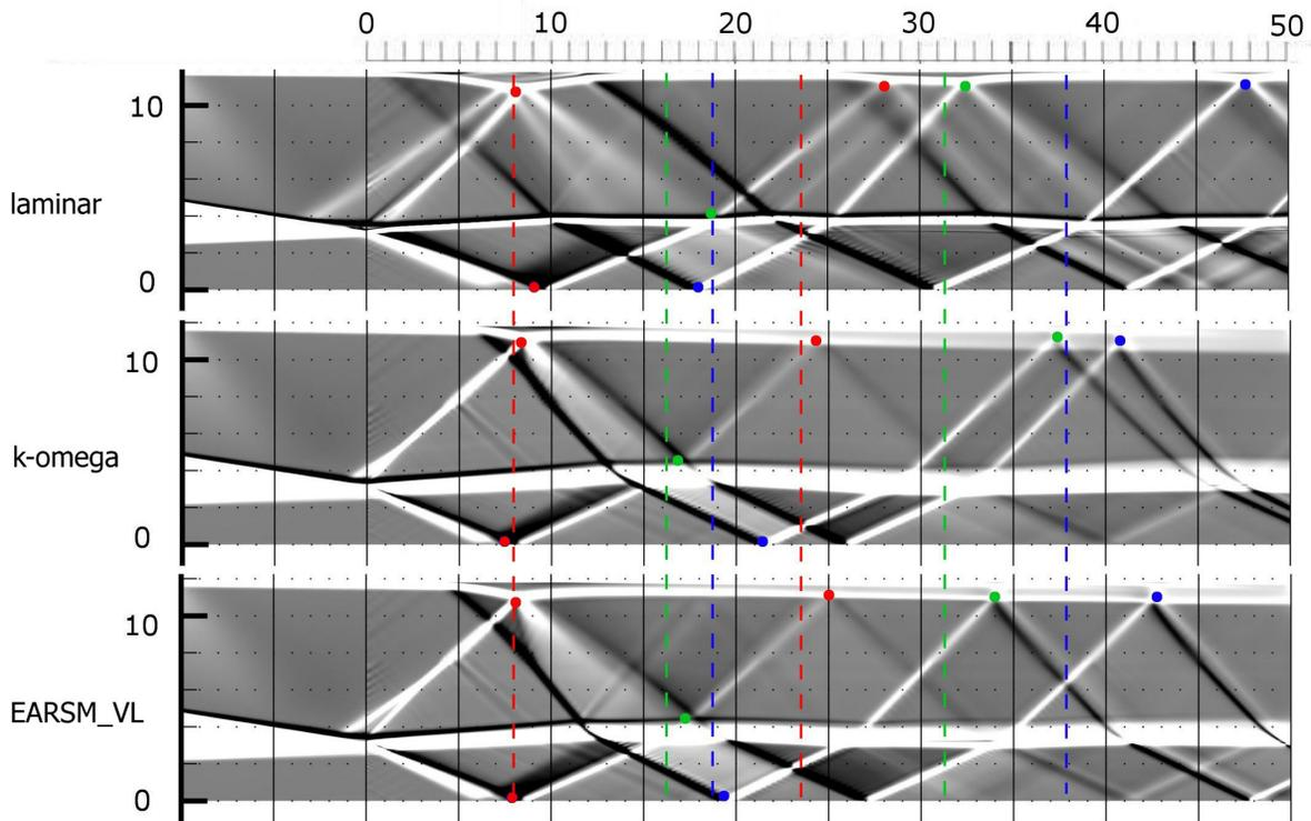
Figure 4: Derivative of density in vertical direction, obtained by computation. The first example is a laminar flow, second  $k - \omega$  (Kok, Vijayasundaram scheme int turb. model), third EARSM (Van Leer scheme in turb. model). Dashed lines show positions of significant points from experiment (Dvořák V., Šafařík P. [1]).
