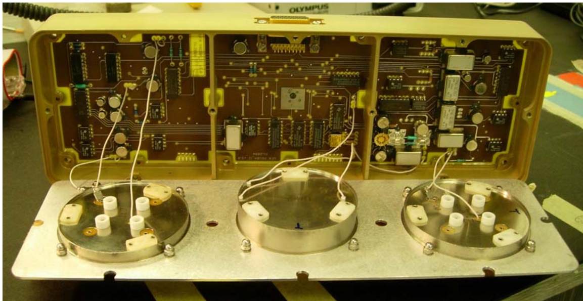
Fig.2. TPMU board and top plate with sensors
