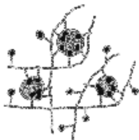
Figure 5 Physical crosslinks in the epoxy-POSS networks
