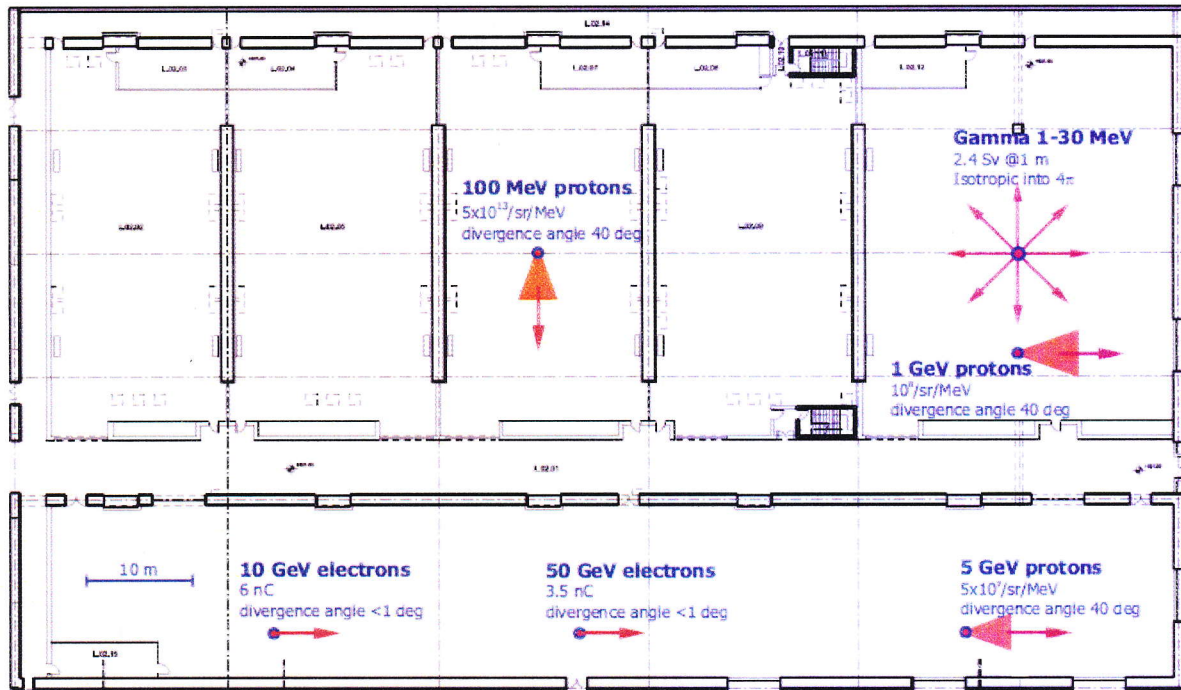
Figure 1. Diagram showing source localizations and directions within the underground floor of the ELI laser building.
