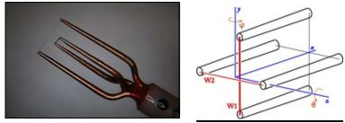
Fig. 2: Cross-sensor probe R521
