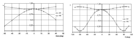
Graph 1a and 1b: Directional characteristics of probe R521 - x-axis is parallel to the flow
