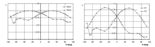
Graph 4a and 4b: Functions  $E^2/E_{max}^2$  (left) and directional characteristics (right) of probe R511 *x*-axis is parallel to the flow
