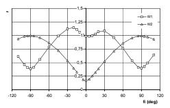
Graph 2: Directional characteristics of probe R521 - x-axis is perpendicular to the flow
