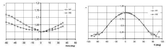
Graph 3a and 3b: Directional characteristics of probe P711 - x-axis is parallel to the flow
