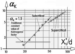
Fortunately, the present approach of evaluating the turbulence parameters by the fitting to the one-equation model solution – such as in Fig. 2 – makes the determination quite easy. The application to the synthetic jet in Fig.3 has shown, for example, the interesting variability of the Kolmogorov factor – again with different trends in the sub- and supercritical regimes.
