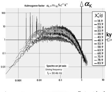
**Fig. 3** Compensated presentation of the spectra measured on the synthetic jet axis. If the law eq.(1) were valid everywhere, the plotted values would be constant independent of the wavenumber k (here related to the microscale y, eq.(2)).
