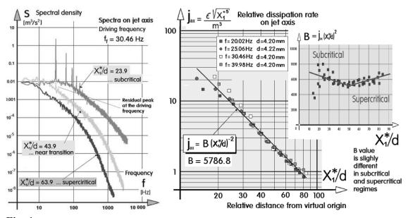
**Fig. 1** (Left): Three examples of one-dimensional velocity spectra measured on the axis of a synthetic jet. The dominance of the coherent oscillation (with harmonics) in the subcritical regime is immediately apparent. **Fig. 2** (**Right**): Relative values of the turbulence dissipation rate on the synthetic jet axis evaluated by applying the expression derived in [5] for two-equation model of turbulence.
