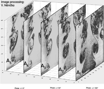
Fig. 3 (Left) Image acquisition synchronised with the excitation makes possible study of the progressive phases of the structure development. In this example of a sequence at increasing phase angle, it may be interesting to follow the vertical motion and growth of the section through the vortex from  $A_1$  to  $A_5$ .
