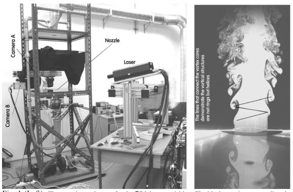
Fig. 1 (Left): The experimental setup for the PIV data acquisition. The black curtains surrounding the jet are here lifted to reveal the nozzle exit. Fig. 2 (Right): A typical example of the investigated jet: Re =  $8.0 \ 10^3$ , excitation frequency 62.8 Hz (Both photographs: P. Antoš)
