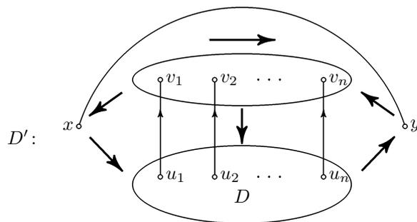
Figure 9. An oriented graph  $D'$  containing  $D$  as its  $k$ -strong periphery
