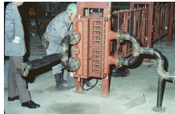
OTEC – Ocean Thermal Energy Conversion (1980-2) Test Plant – 500 TEG modules [Uemura, ITTJ]
