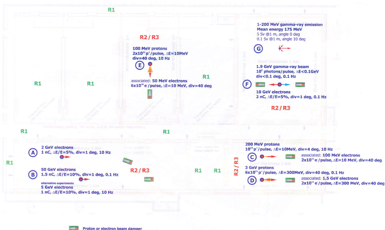
Figure 2. Diagram showing localization of the secondary sources and emission directions within the basement of the ELI laser building.
