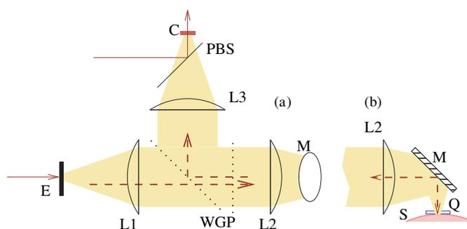
**Figure 1.** Schematics of the THz beam path in the experiment. (a) top view, (b) side view. E: THz wave emitter, L1–L3: lenses, WGP: wire grid polarizers, M: mirror, Q: quartz window, S: skin sample, PBS: pellicle beam splitter, C: electro-optic crystal (THz sensor). The thin solid lines with arrows represent the path of the laser pulses.
