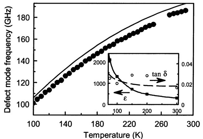
Fig. 2. Tuning curve of the defect mode. Filled circles, measured defect frequency; solid curve, results of a numerical simulation. Inset, temperature dependence of the permittivity ( $\epsilon$ ) and the loss tangent ( $\tan \delta$ ) of a SrTiO<sub>3</sub> single crystal at 0.2 THz measured by time-domain THz spectroscopy. Points, measured values; curves, analytical fits of the data.
