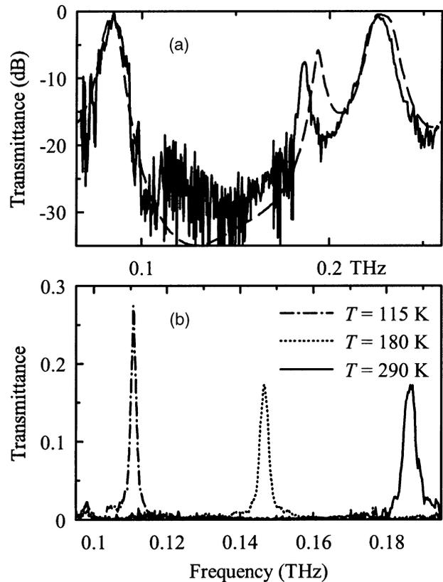
Fig. 1. Power transmittance of the investigated structure. (a) Room temperature: solid curve, experiment; dashed curve, numerical simulation. (b) Typical spectra experimentally obtained in the tuning range.
