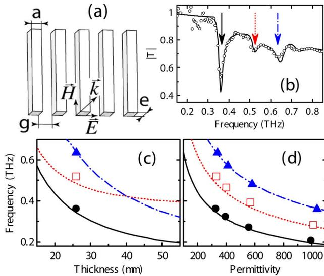
Fig. 1. (Color online) (a) Geometry of the MM structure. (b) Measured and calculated transmission amplitude spectra of the studied sample at room temperature. Mie resonances are indicated by arrows. (c) Resonant frequencies as a function of the thickness  $e$ . (d) Resonant frequencies as a function of  $\text{Re } \epsilon$  of the rods. Symbols, experiment; lines, calculations. The resonance indicated by the dash-dotted curve has a nonmagnetic character.
