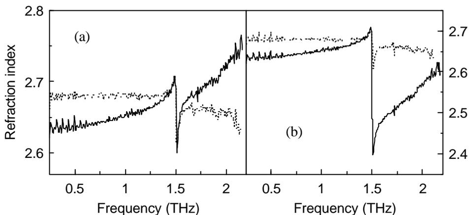
FIGURE 3 Refraction index of LGO. Solid lines:  $n$  calculated from transmission function using equation (2); dotted lines:  $n$  calculated from  $\kappa$  through KK relations. Phase branch choice following the notation of Figure 2: (a) long-dashed line, (b) short-dashed line.
