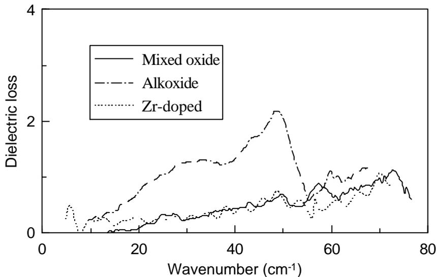
FIGURE 5 Dielectric losses of BMT ceramics obtained by TDTS.
