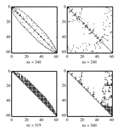
*Fig. 1.* Example of matrix structure after reordering (top) and after factorization (bottom) Reverse Cuthill-McKee ordering (left) and Minimum Degree ordering (right)
