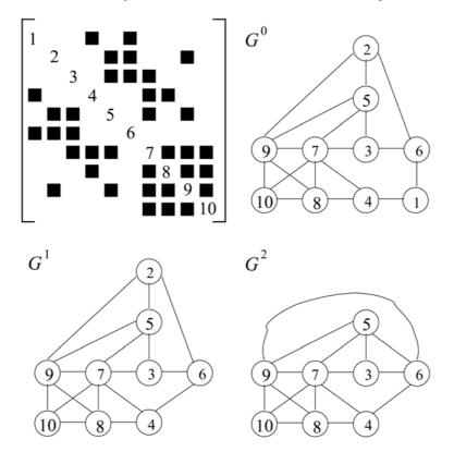
Fig. 2. Example of matrix and its elimination graph (initial and after first two steps)
