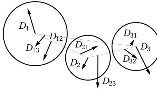
Figure 2: First  $D_i$  and second  $D_{ij}$  groups of dipoles,  $N = 3$ . Dipoles are denoted by the arrows, their lengths are proportional to the strengths of dipoles (for good orientation the lengths of arrows of the second group are magnified five times).
