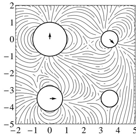
Figure 4: Streamlines for flow past four moving cylinders.
