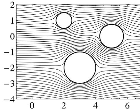
Figure 3: Streamlines for uniform flow past three stationary cylinders.
