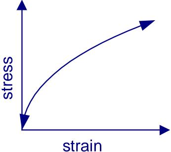
For large displacements (but small strains) engineering strain (Cauchy) is replaced by **Green-Lagrange strain** and engineering stress is replaced by **2PK stress** and **TL** or **UL** formulations should be used
