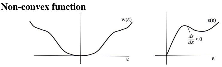
if  $ds/d\varepsilon_x < 0$  (locally) then  $s(\varepsilon_x)$  is not motonically increasing strain energy function is non - convex material is said to exhibit strain softening
