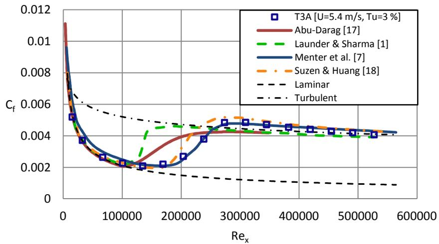
Figure 3: Predicted skin friction coefficient in transitional boundary layer subjected to moderate turbulence intensity
