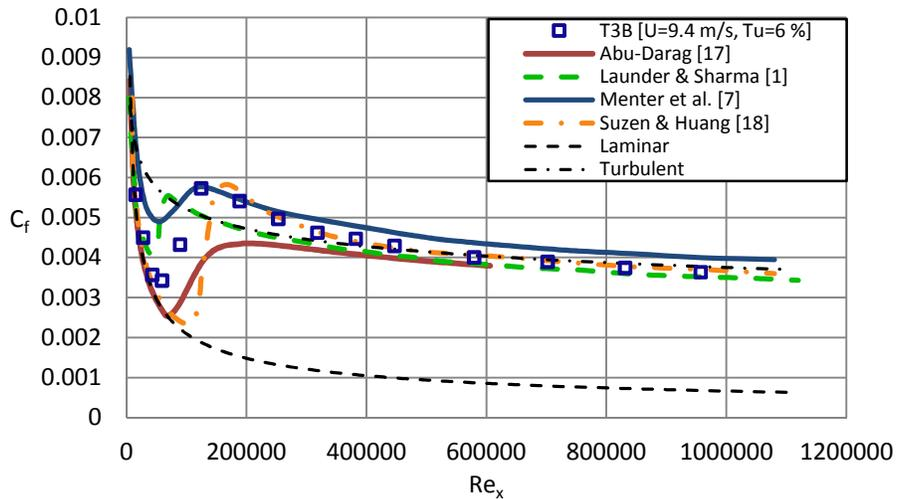
Figure 4: Predicted skin friction coefficient in transitional boundary layer subjected to high turbulence intensity
