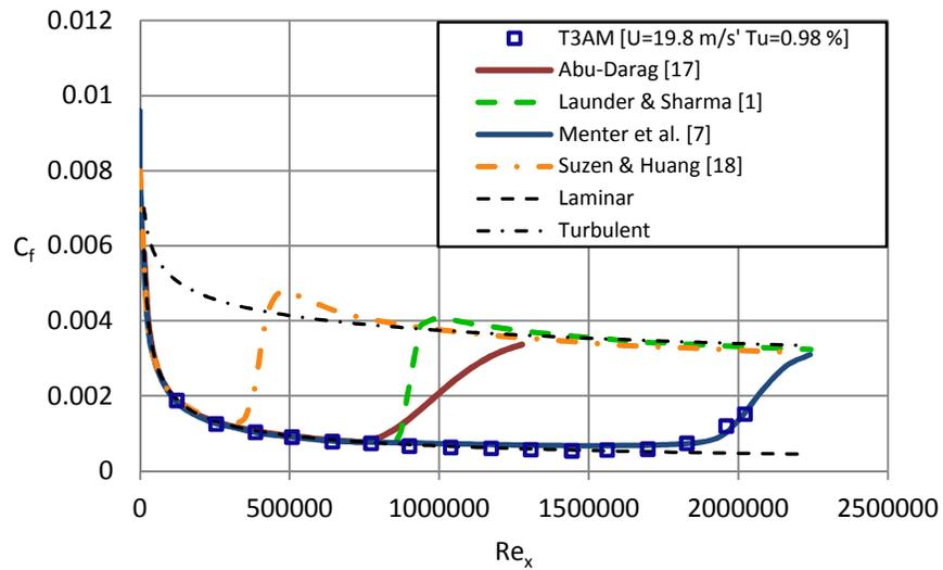
Figure 2: Predicted skin friction coefficient in transitional boundary layer subjected to low turbulence intensity
