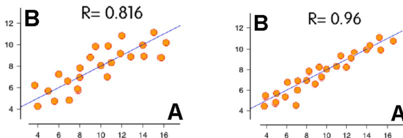
**Figs. 6, 7** Two examples of the correlation coefficients  $R$  computed for two  $5 \times 5$  data values in the vectors **A** and **B**. The value  $R$  is interpreted as the measure of the scatter in the mutual linear dependence of the two vectors.
