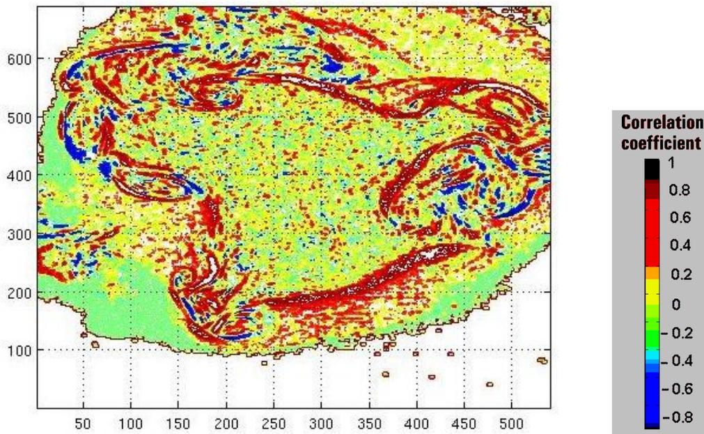
**Fig. 8** An example of the cross-section image colour-coded by the local values of the magnitude of correlation coefficient evaluated for  $5 \times 5$  sub-images. The red colour indicates the contours of vortical coherent structures. The absence of structures in the central part of the cross section is the consequence of the shear-less “potential” core of the jet.
