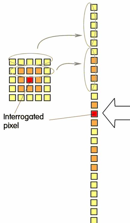
**Fig. 5** The formation of the vectors **A** and **B** from the neighbouring pixels. Alternative choices are possible, whereby the procedure can either suppress or enhance some directions of motion in the interrogation plane..
