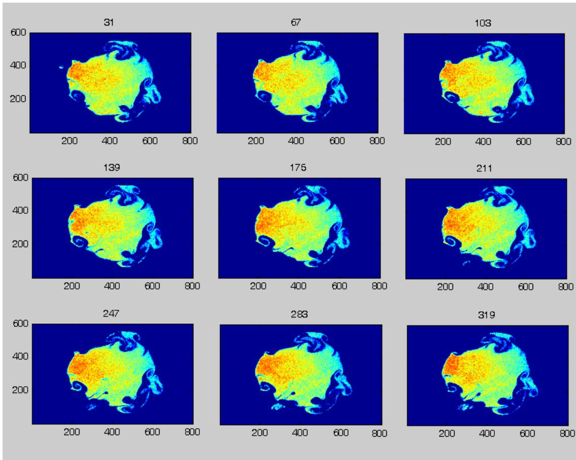
**Fig. 3** Typical examples of cross-section images recorded in the same phase of the harmonic triggering. This sample of nine images demonstrates the performance of triggering signal generator designed and built by Mr. M. Pavelka. Intensity of scattered light corresponds to the local density of water droplets concentration.
