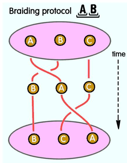
**Fig. 16** Full braiding motion: the hair plait consists of objects positioned by repeated braiding following the same protocol.
