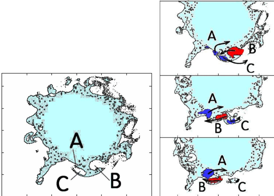
**Fig. 10 (left):** Typical boundaries evaluated by the posterisation procedure. The vortical objects are here presented as empty voids. **Fig. 11 (right)** The braiding motion of the vortices in the outer, mixing region of the jet, made more apparent by filling with blue and red colour. The pictures were taken after full 360 deg phase shifts..
