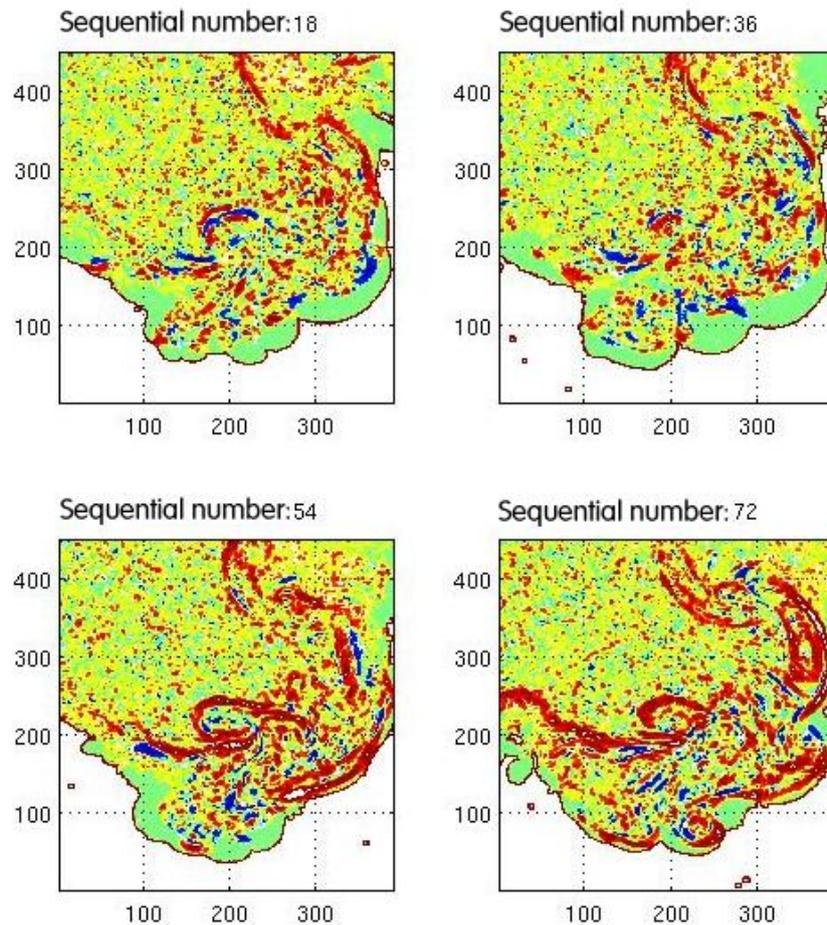
**Fig. 9** A detail of an example of the jet cross section, evaluated in different phases of the harmonic excitation. The colour coding by the value of the correlation coefficient shows by the red colour of high  $R$  the boundaries of the interacting vortical object, seen in inclined cross sections. .
