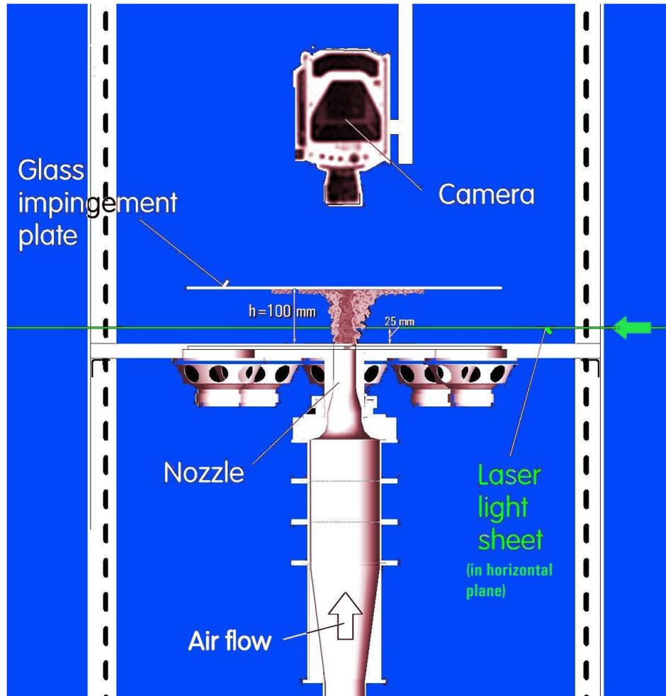
**Fig. 1** The experimental facility, shown in meridian section. The air jet generated in the nozzle impinges upon the glass plate. The apparent cross section through the jet is made by the “laser knife” at the distance  $0.25 h$  from the nozzle and is recorded by the camera hidden behind the impingement plate.
