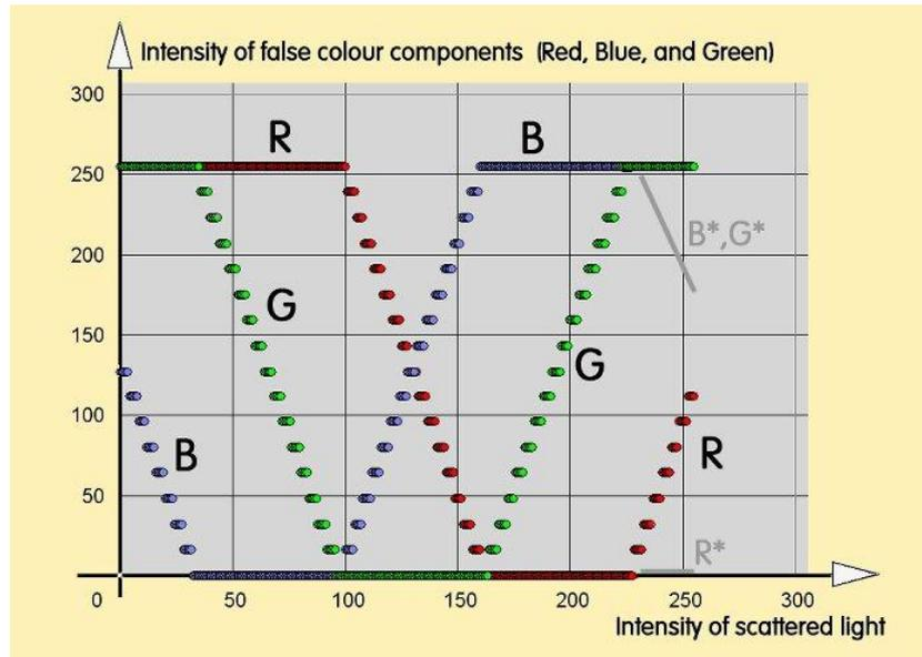
Fig. 4 Conversion diagram used for false-colour presentation grey-scale intensity images. It was used to obtain the images in Fig. 3. For symmetry of the function, the red component intensity  $R$  here rises at the blue end of the colourbar while  $B$  and  $G$  intensities remain high. A better appearance may be obtained with the suggested alternative, marked with asterisks.
