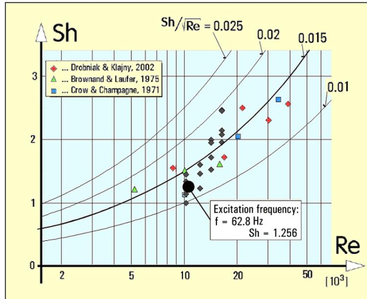
**Fig. 2** Dependence of Strouhal number  $Sh$  of natural instabilities in the mixing layer (computed from the vortex convection velocity  $w_c$ ) on Reynolds number  $Re$  computed, as usual, from the the nozzle exit velocity  $w_e$ ). This diagram was used to adjust the excitation frequency.
