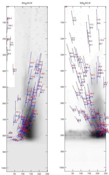
Fig. 3. Two perpendicular images with found velocity and acceleration vectors.
