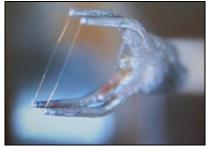
Fig.2: Photo of long-wire parallel-sensor probe
