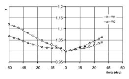
Graph 1a and 1b: Directional characteristics of probe P711 - x-axis is parallel to the flow
