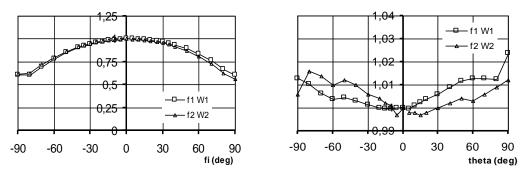
Graph 2a and 2b: Directional characteristics of probe P712 - x-axis is parallel to the flow
