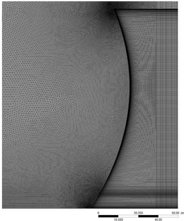
Fig. 1. Detail of the computational mesh
