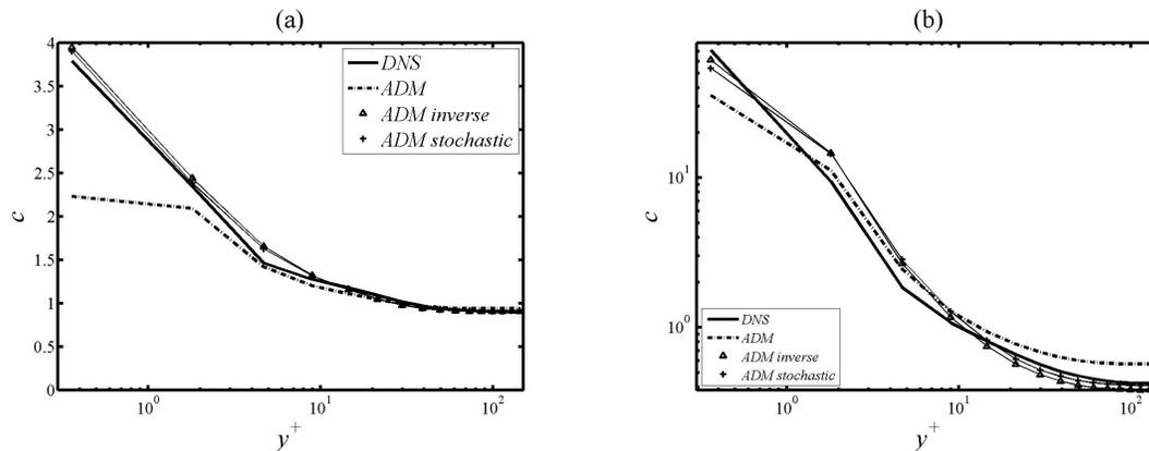
Figure 4: Concentration of particles close to the wall in the stationary state for (a)  $St=1$  and (b)  $St=5$
