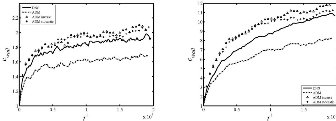
Figure 3: Concentration of particles close to the wall as a function of time for  $St=1$ ,  $St=5$ .
