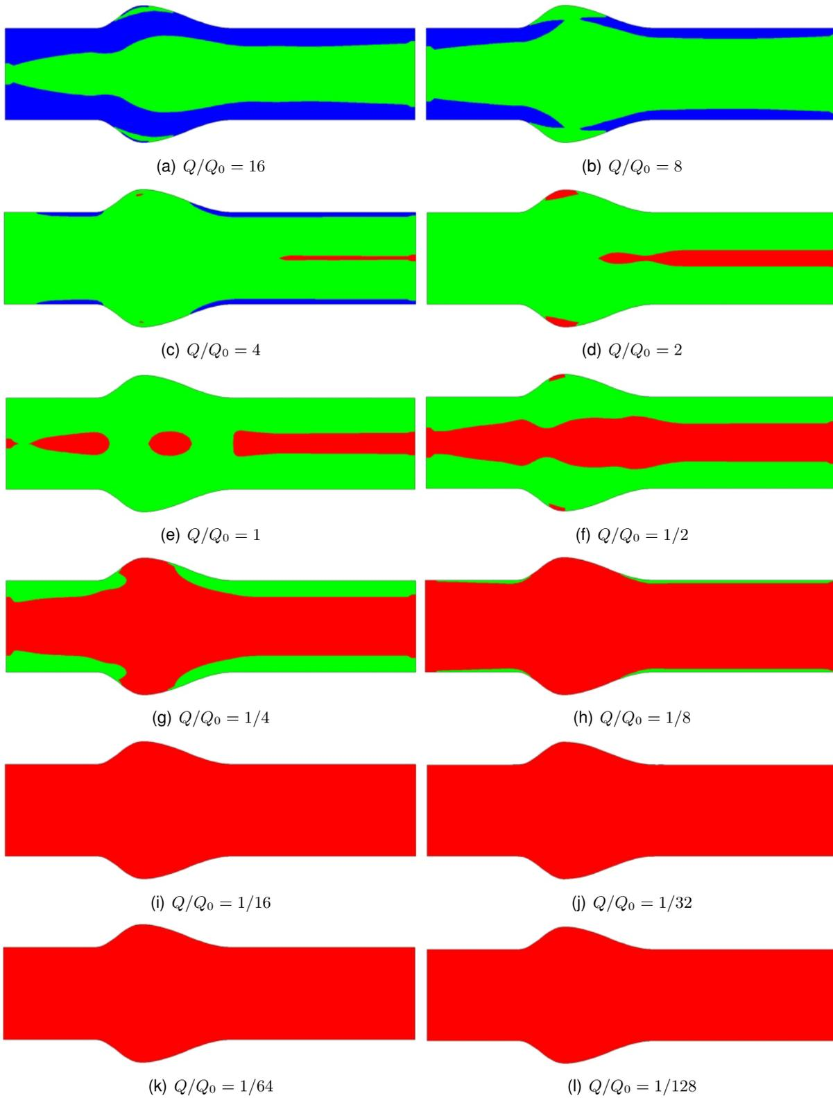
Figure 2: Relative viscosity magnitude,  $\bar{\eta} = (\eta(\dot{\gamma}) - \eta_{\infty})/\eta_{\infty}$ , aneurism geometry
